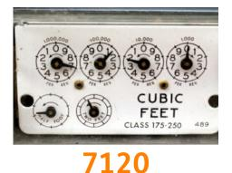
Some meters may have dials. To read these meters, start on the left. See the number that the pointer has just passed. The meter here reads **7120**.
