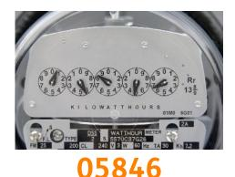
When reading an electricity meter, you should always end up with 5 numbers.
